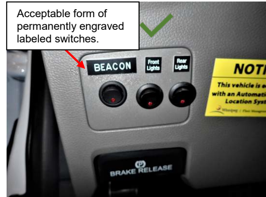
Picture above shows example of permanent engraved label switches.
